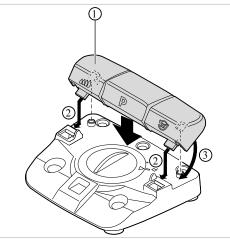
Plug the button bar ① onto the foot control ② and press it on lightly until the button bar ① snaps into place ③.
