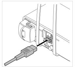
Plug the mains cable first into the mains plug on the device and then the other end of the mains cable into the electrical outlet of the supply mains.
