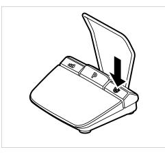
The direction of motor rotation can be changed during the treatment using the direction of motor rotation key of the foot control. The changed direction of motor rotation is shown on the display. For safety reasons, running in counterclockwise direction is not saved.
