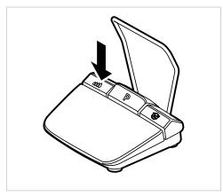
The coolant flow can be set during the treatment using the pump key of the foot control. The changed value is shown on the display and is then available for the next use.
