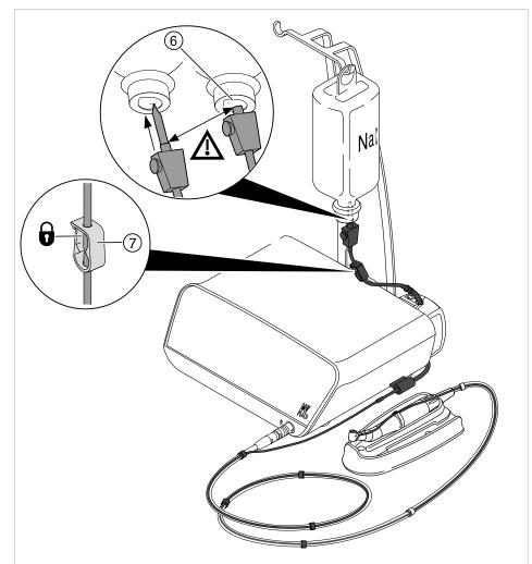
Stick the puncture needle (6) into the coolant container and hook-in the coolant container on the bottle holder.
