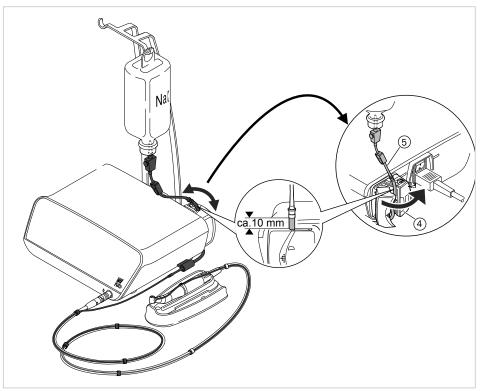
• Open the lock ④ and insert the pump hose ⑤.
