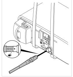
Insert the plug of the foot control in the electrical outlet for the foot control. Make sure that the marker arrows on the plug and the socket are aligned towards each other.
