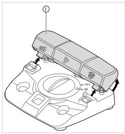
Pull the button bar ① including the pump button, program button, and motor direction button slightly upwards and take it off the foot control. 7 Reprocessing steps in accordance with DIN EN ISO 17664 | 7.1 Cleaning
