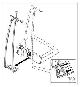
Press down the click-stop knob on the bottom side of the unit and pull off the bottle holder ① towards the back.
