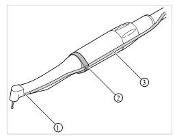
Route the coolant hose ③ from the unit along the motor cable (clips) and connect it to the straight or contra-angle handpiece ④. Place the coolant hose ③ into the holding ring ② for this purpose.
