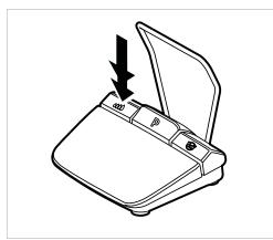
Press the pump key on the foot control for an extended time.
