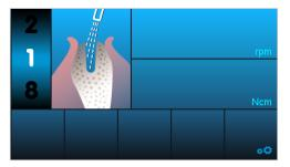
The rinsing function serves to feed liquid and to start-up the illumination on the handpiece. The motor is not activated during this process. The rinsing function can be called up manually at any time.
