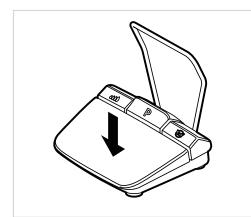
Press the speed key on the foot control to start the rinsing function and control the coolant flow.
