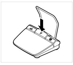
The program steps can be selected during the treatment using the program key of the foot control. After the last program step follows the first step again. Press the program key long to select the previous program step.
