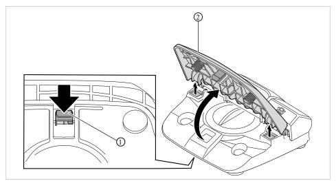
► On the underside of the foot control, press down the snap-in lug ① of the speed button ② and take the speed button ③ off the foot control.
