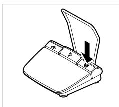
Press the direction of motor rotation key of the foot control to set the direction of motor rotation.
