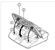
Plug the speed button ① onto the foot control and press it on lightly until the snap-in lug ② snaps in. Make sure that the pedal springs are situated in the recesses of the housing ③.
