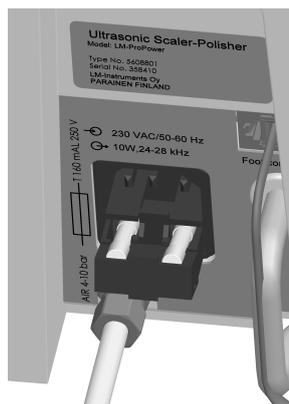
3. Inspect the fuses for damages. Replace damaged fuses with new ones. Verify the fuse specifications according to the Technical data section on page 28.
