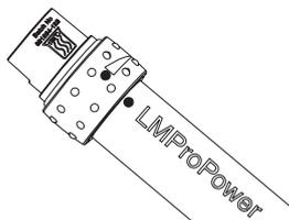
3. Squeeze the ErgoGrip gently at the top and at the same time slide it off the handpiece. Do not squeeze too hard at the ErgoGrip as this can make the removal difficult.
