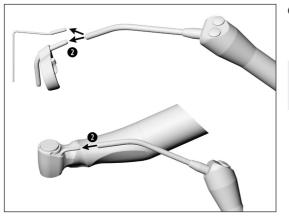
② Blow through the coolant tube and coolant outlets with the air syringe.
