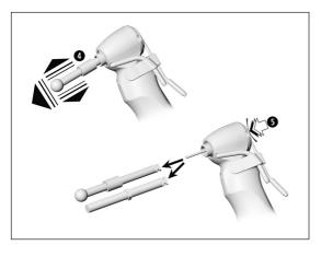
Check secure location by applying slight axial tension.
